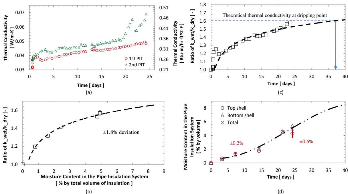
**Figure 5:** Test results on phenolic pipe insulation systems: a) thermal conductivity variation with time b) thermal conductivity ratio ( $k_{wet}/k_{dry}$ ) with moisture content; c,d) ratio and moisture content with time
