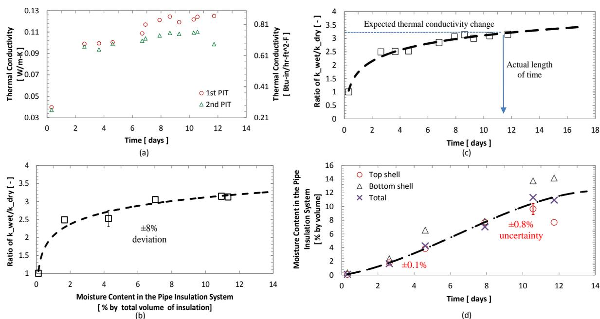
**Figure 2:** Test results on fiberglass pipe insulation systems: a) thermal conductivity variation with time b) thermal conductivity ratio ( $k_{wet}/k_{dry}$ ) with moisture content; c,d) ratio and moisture content with time
