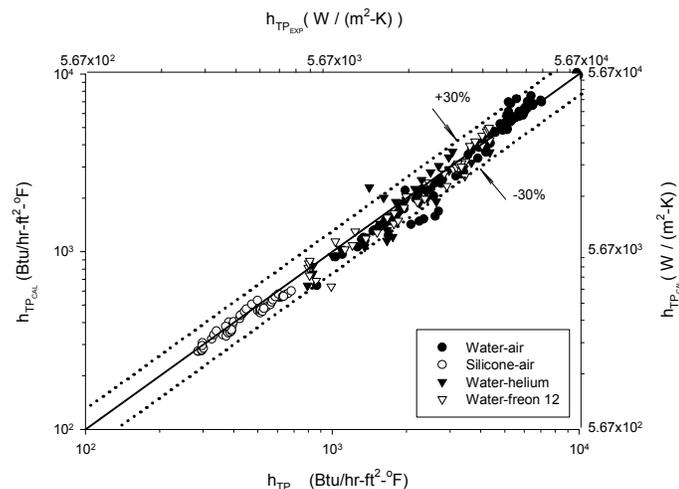
Figure 1 Comparison of the new correlation [Equation (1)] with all of the two-phase heat transfer experimental data (255 data points).
