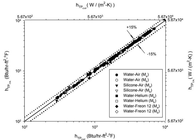
Figure 3 Comparison of the correlation using ANN with all of the two-phase heat transfer experimental data (255 data points).
